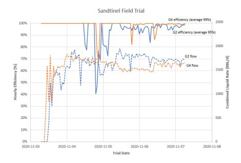
This curve shows both the hourly flow rates measured for each parallel sand separator, as well as the measured hourly efficiency of sand removal via upstream and downstream sampling. The separation efficiency of the G2-S Defender was 95% sand removal over the course of the trial; the separation efficiency of the G4-S Maverick was over 99% sand removal. Both separators saw approximately the same amount of sand, approximately 2,900 lb of sand per day each, with hourly dump operations performed.
