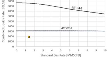
This operating curve shows the estimated envelope where the Sandtinel sand separators will provide best in class sand separation efficiency, beyond any other mechanical separator on the market. While inside this curve, our partner was guaranteed to be able to see at least 95% separation efficiency. However, reports from the field for the next generation Maverick G4-S were a sand removal efficiency of **over 99%** (only ~60 lb of carryover per day).
